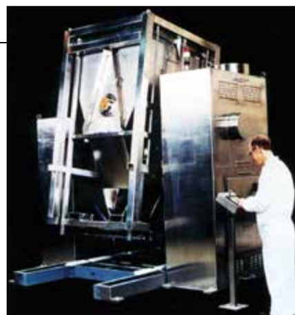
FIGURE 2. With tumbling in-bin blenders, the storage container itself becomes a blender
