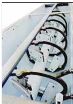
FIGURE 3. Paddle (left) and ribbon (right) blenders are convection-type units
