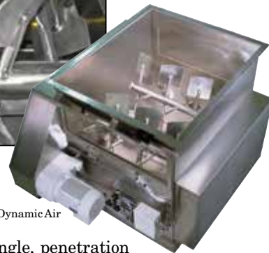
FIGURE 7. These high-shear mixers combine fluidization and convective features
