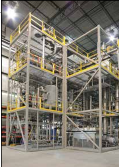
FIGURE 3. Here, a modular shale-oil upgrading demonstration plant is in the shop
