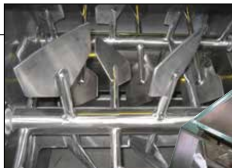
FIGURE 7. These high-shear mixers combine fluidization and convective features
