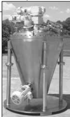
FIGURE 5. A conical screw, or Nauta-type mixer is commonly used for cohesive powder blending
