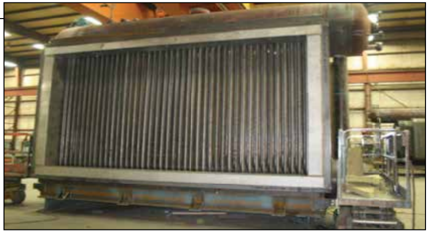
FIGURE 2. A cross-flow boiler with finned tubes (left) is very compact, while a longitudinal gas boiler with plain tubes (right) has a large footprint
